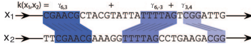
Fig. 1. Given two sequences x_1 and x_2 of equal length, the WD kernel with shift consists of a weighted sum to which each match in the sequences makes a contribution \gamma_{k,p} depending on its length k and relative position p , where long matches at the same position contribute most significantly. The \gamma 's can be computed from the \beta 's and \delta 's in (2). The spectrum kernel is based on a similar idea, but it only considers substrings of a fixed length and the contributions are independent of the relative positions of the matches to each other.
