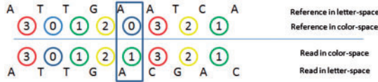
Fig. 1. Translating the read from color-space to letter-space may result in a new sequence different from the original read if there exists a color-space error.
